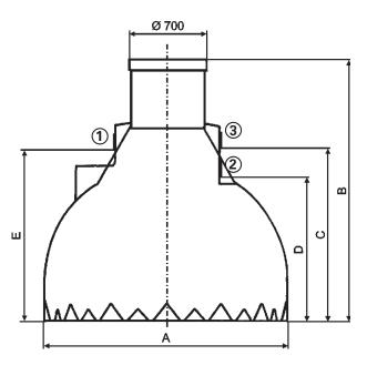
Infiltra-Installation Technical tion/drain Rainwater Diameter depth B Volume conductions connection inlet Art.-No. Α C D Ε RS 1000/RS 1010 Ø 2150 4 m<sup>3</sup> 2340 1580 1375 1550 (1,000/gallons) (7 ft.) (7.7 ft.) (5.1 ft.) (4.5 ft.) (5.1 ft.) Ø 2350 2480 1645 1360 1600 RS 2000/RS 2010 5 m<sup>3</sup> (1,300/gallons) (7.7 ft.) (8.1 ft.) (5.4 ft.) (4.5 ft.) (5.3 ft.) RS 3000/RS 3010 Ø 2350 2730 1910 1610 1850 6 m<sup>3</sup> (1,500/gallons) (7.7 ft.) (8.9 ft.) (6.3 ft.) (5.3 ft.) (6.1 ft.)
